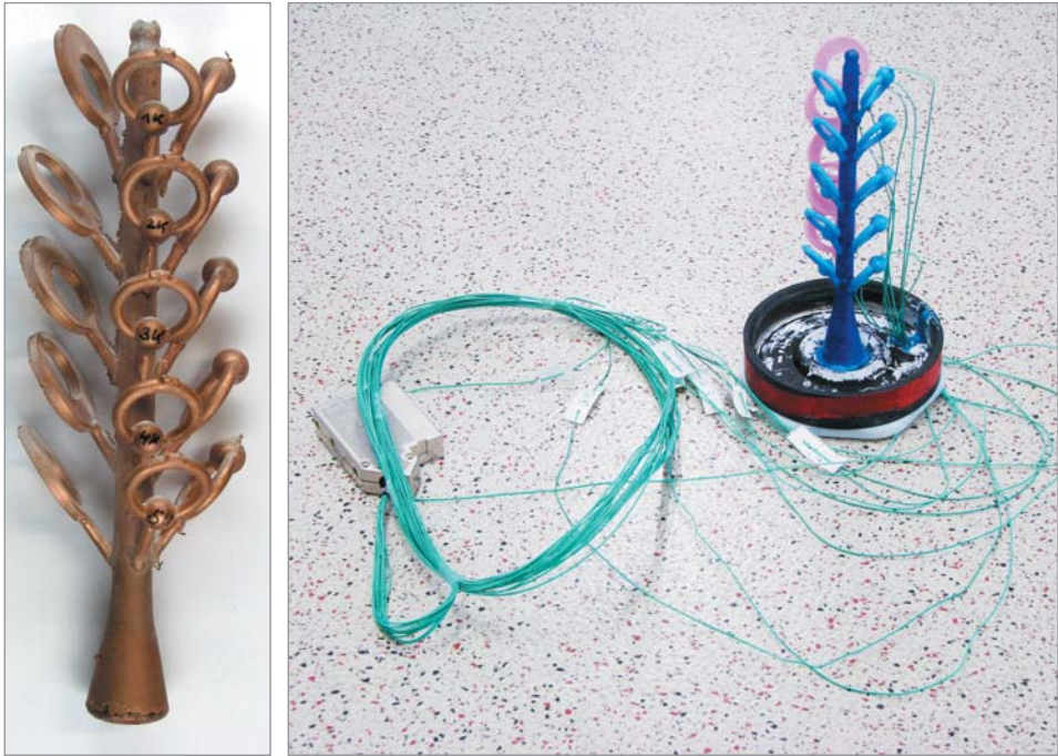
Figure 3 Left: as-cast 18K red gold tree after devesting; right: wax tree with set of thermocouples
